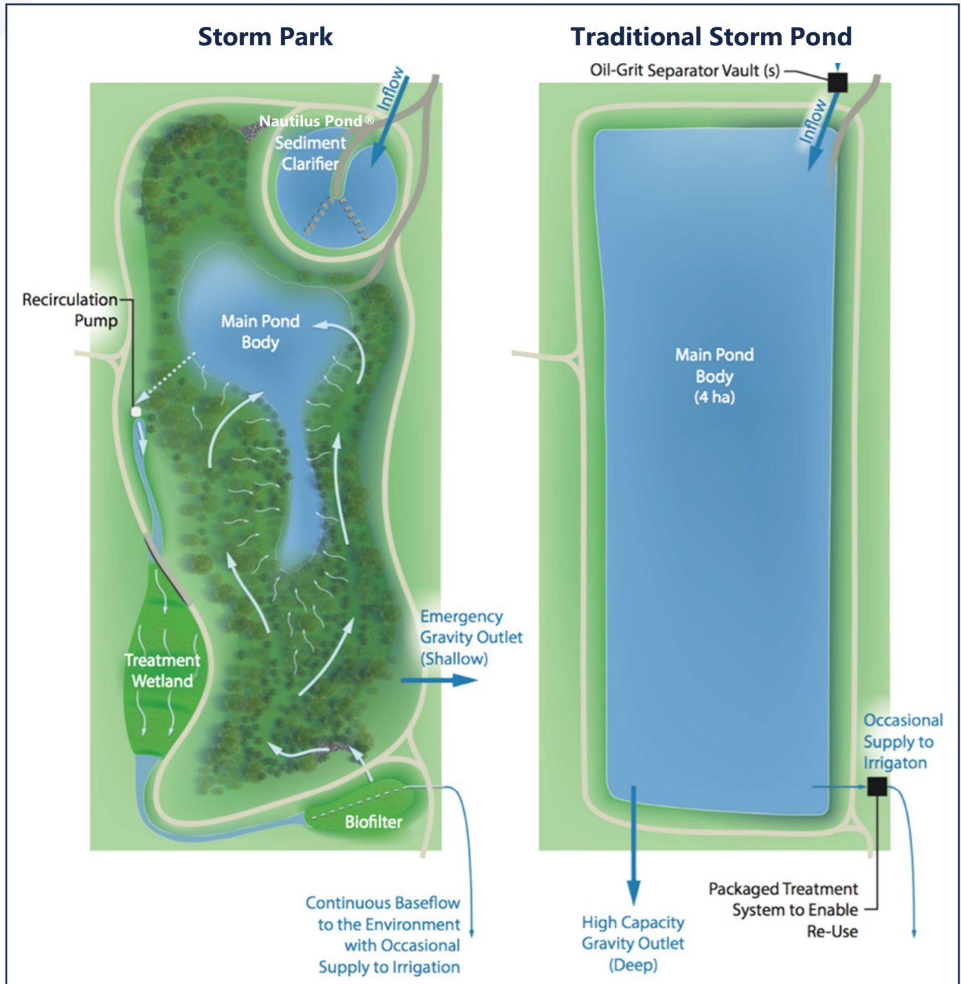
Figure 5.4: Storm Park vs. Traditional Storm Pond
