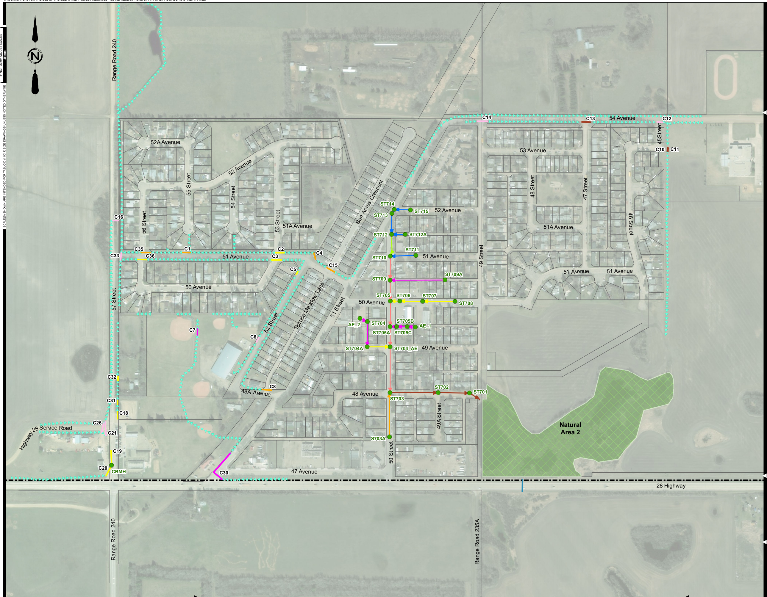
FIGURE No. 3-2 TOWN OF BON ACCORD STORM MASTER PLAN UPDATE EXISTING STORMWATER SYSTEM
