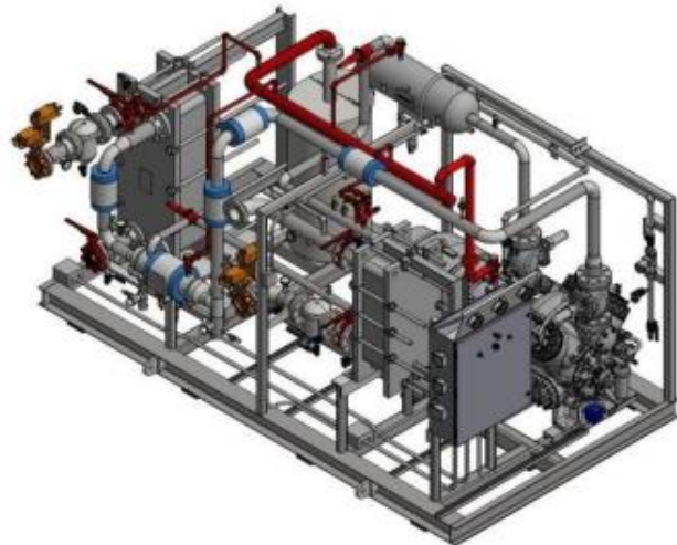
Figure 9 - Refrigeration Skid Package
