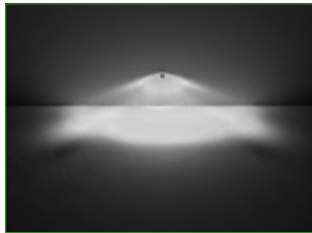
Type 2 Designed to IES Type II classification.
