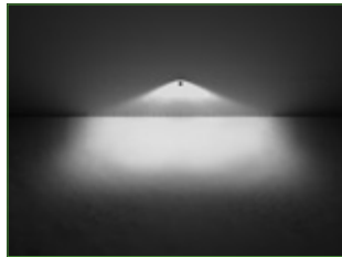
Type 3 Designed to IES Type III classification.
