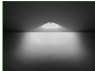
Type 4 Designed to IES Type IV classification.
