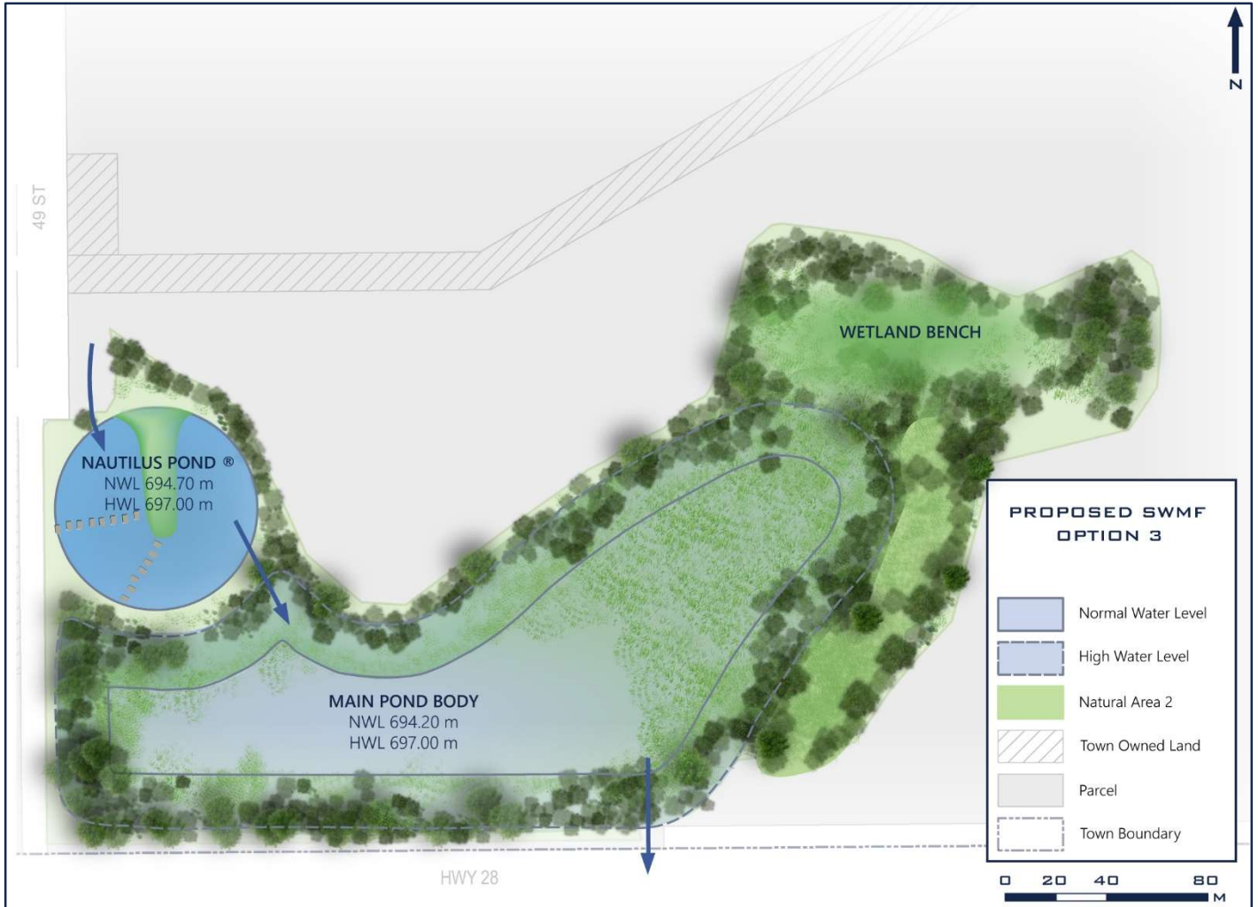
Figure 5.6: Storm Park (without Treatment Cells) Site Plan
